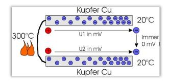
Figure 2: "Thermocouple" consisting of two identical metals (Cu)
