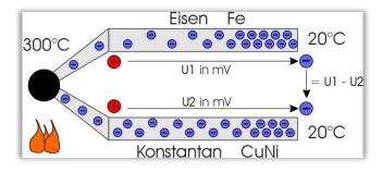
Figure 3: Thermocouple made of iron - constantan (FeCuNi)
