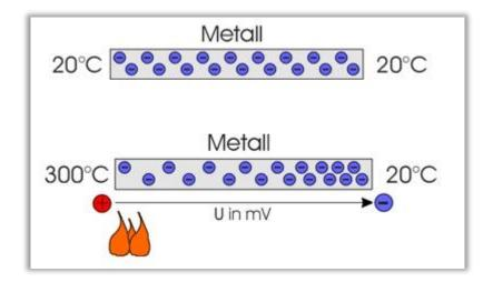
Figure 1: "Electron migration" due to heating
