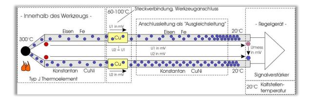
*Figure 4: Thermocouple with connector and compensating cable*
