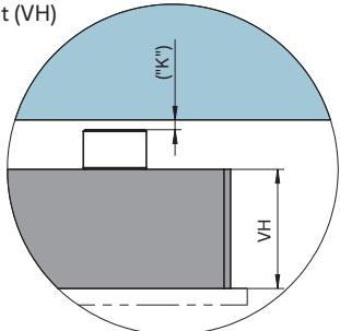
Dimension "K" required for heat expansion is to be ensured by grinding the pressure pad (12 + 0.1 mm)! Determine the difference between the height of the manifold system and the height of the frame plate when installed!  $\Delta T$  specifies the temperature differential between the processing temperature and the mould temperature!
