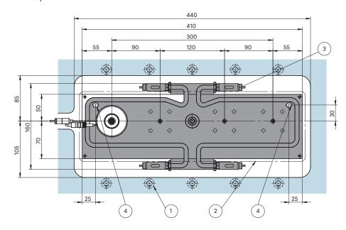
DS Edge distance: a. min. 35.0 with nozzle size  $\leq 6$ b. min. 45.0 with nozzle size 8 or 10 c. min. 50.0 with nozzle size  $\geq 12$
