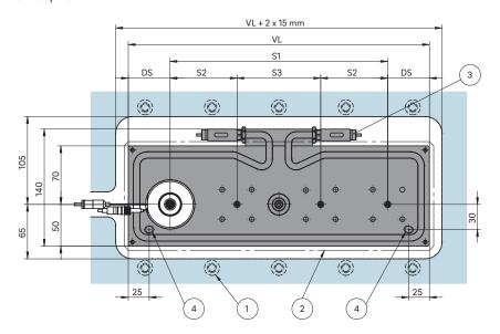
DS Edge distance: a. min. 35.0 with nozzle size  $\le 6$ b. min. 45.0 with nozzle size 8 or 10 c. min. 50.0 with nozzle size  $\ge 12$
