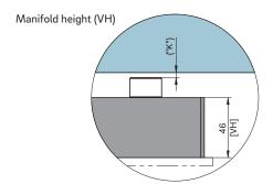
Dimension "K" required for heat expansion is to be ensured by grinding the pressure piece (12 + 0.1 mm)! Determine the difference between the height of the manifold system and the height of the frame plate when installed!  $\Delta T$  specifies the temperature differential between the processing temperature and the mould temperature!
