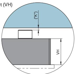
Dimension "K" required for heat expansion is to be ensured by grinding the pressure pad ( $12 + 0.1 \text{ mm}$ )! Determine the difference between the height of the manifold system and the height of the frame plate when installed!  $\Delta T$  specifies the temperature differential between the processing temperature and the mould temperature!
