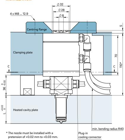
Cross section C-C: recess for nozzle head and connection hoses
