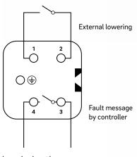
Lowering input/ fault signal output
