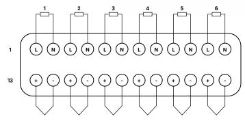
Load and thermocouple connector
