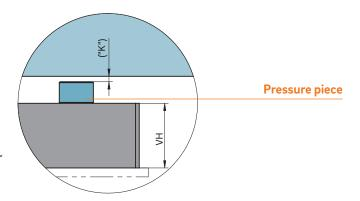
The size "K" required for heat expansion is to be ensured by grinding the pressure pad (12 + 0.1 mm)! Determine the difference between the height of the manifold system and the height of the frame plate when installed!  $\Delta T$  specifies the temperature differential between the processing temperature and the mould temperature!
